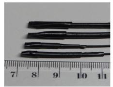
Fibre sensors for in vivo dosimetry during radiotherapy - S. Lomazzi
